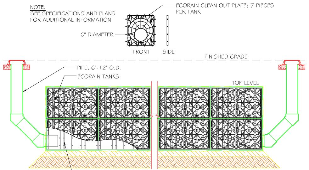
CUTAWAY VIEW CLEANOUT ACCESS W/CLEANOUT PLATE SIDE ELEVATION, TYPICAL BOTH SIDES, REFER TO CLEANOUT PLATE ELEVATION ABOVE
